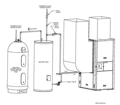
Figure 7A – Desuperheater, Single Tank Concept
