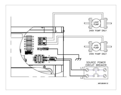
**Disconnect** – field provided external safety disconnect is required, see nameplate max amps.
