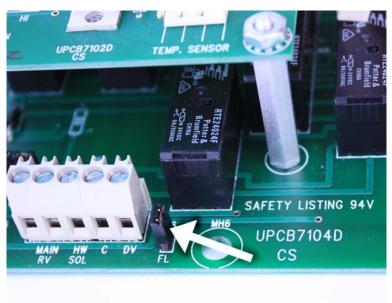
Comment – factory default is set up for HW (hot water) to activate the compressor at Full Load. If sizing is such that Part Load compressor (first stage) only is required for the hydronics mode, remove the jumper peg from the control board in the location labeled "FL" as shown here . If there is an external aquastat with stage 1 and stage 2 capability, call factory for wiring instructions.
