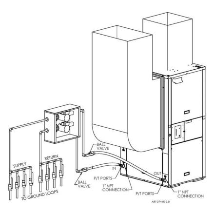
Figure 4 – Pressurized Closed Loop with Flow Center – Typical piping arrangement.
