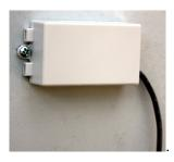
**Outdoor Sensor (OT)** – extend sensor to an outdoor location properly sampling the outdoor temperature. Select a location away from direct sunlight and where the sensor will not pick up false temperature from the heat pump outdoor unit, refrigerant line sets, dryer vent, reflection off of steel siding, etc. Do not install the sensor in any type of enclosure, as this will falsely trap and pick up radiant sun temperature. Mount the sensor horizontally on the structure using the screws provided.
